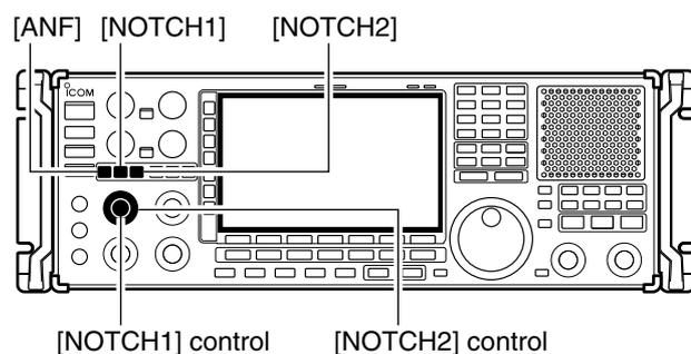
This receiver has auto and manual notch functions. The auto notch function uses DSP to automatically attenuates up to 3 beat tones, tuning signals, etc., even if they are moving. The manual notch can be set to attenuate a frequency via the [NOTCH1]/[NOTCH2] controls.
