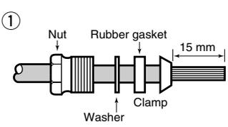
Slide the nut, washer, rubber gasket and clamp over the coaxial cable, then cut the end of the cable evenly.
