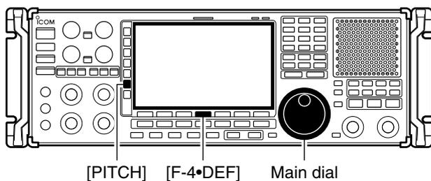
The received CW audio pitch can be adjusted to suit your preference (from 300 to 900 Hz in 5 Hz steps). This does not change the operating frequency.
