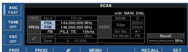
Programmed scan searches for signals within a specified frequency range, using the selected tuning step increments. The result is like 'automatically' rotating of the main dial.
