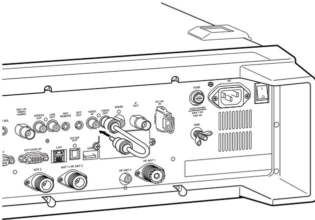
Connect the RCA cable between [VIDEO IN] and [VIDEO OUT].
