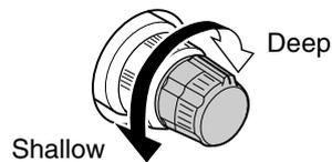
**21 RF GAIN CONTROL [RF]** (outer control; p. 3-8)
