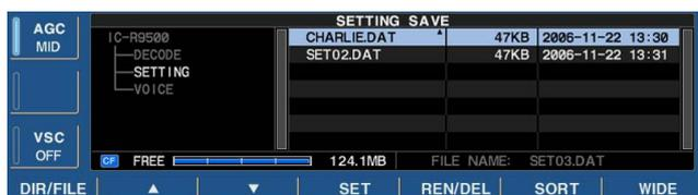
The file name, saved in the CF memory card or USB-memory, can be re-named from the receiver as desired.
