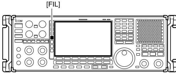
The receiver has 3 passband width IF filters for each mode.
