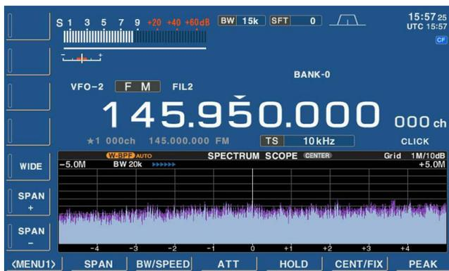
The wide band-pass filter function can change the RF band pass filter and the select the wide band-pass filter
