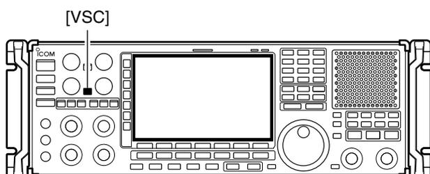
This function is useful when you don't want unmodulated signals pausing or cancelling a scan. When the voice squelch control function is activated, the receiver checks received signals for voice components.
