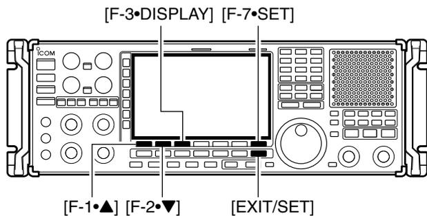
A total of 4 meter types are available in the IC-R9500— S-meter,  $\text{dB}\mu$ ,  $\text{dB}\mu(\text{EMF})$  and  $\text{dBm}$  meters. Follow the instructions below for the meter type selection.
