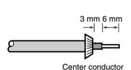
Strip the cable and fold the braid back over the clamp.
