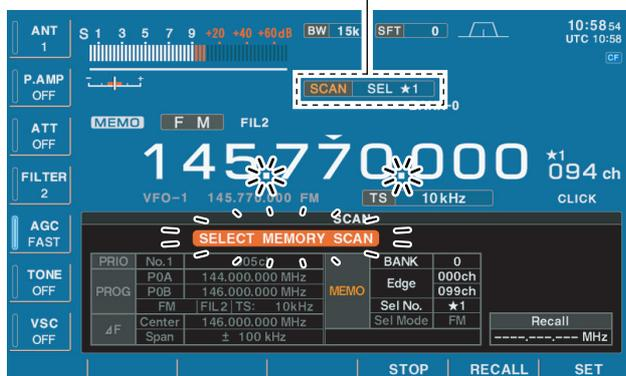
Select memory scan allows you to increase scan efficiency by searching for specified channels group only.
