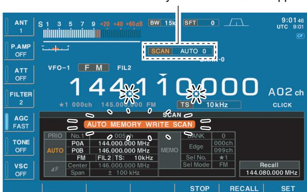
Auto memory write scan operates in the same way as programmed scan. However, when a signal is received, the received frequency is automatically written into a memory channel in the auto write bank (A00–A99).
