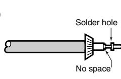
Tin the center conductor. Install the center conductor pin and solder it.
