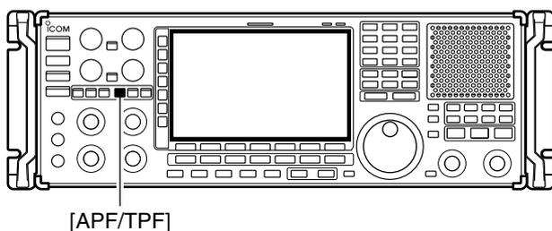
The twin peak filter changes audio frequency response by boosting the mark and space frequencies (2125 and 2295 Hz) for better reception of FSK signals.
