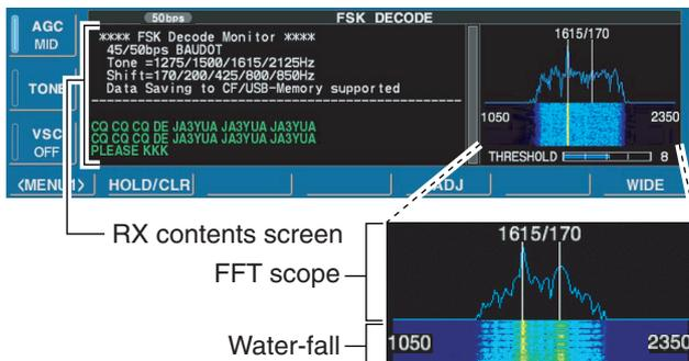
A DSP-based high-quality Baudot FSK decoder is built-in to the IC-R9500.
