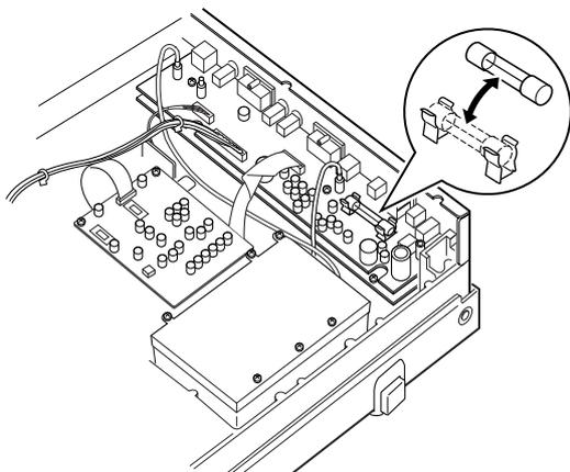
When no external DC output is available from [EXT DC] and ACC connector, the internal fuse may be open. Replace the fuse in this case.
