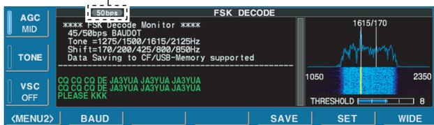
The data transfer rate can be selected from two speeds, 45 bps and 50 bps.
