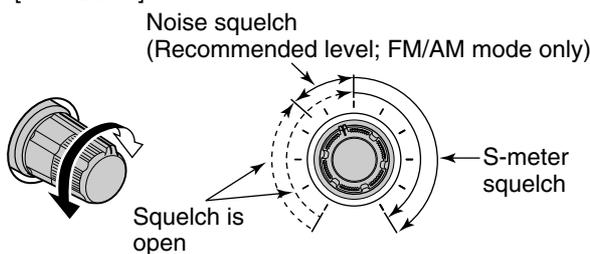
The squelch disables output from the speaker (closed position) when no signal is received.
