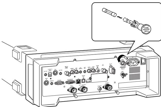
The AC power input fuse is held in the [FUSE] holder.
