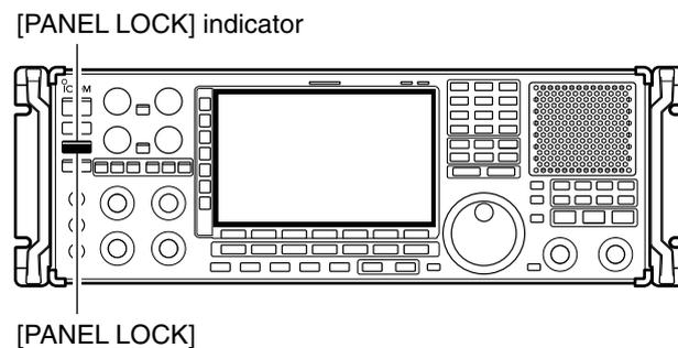
To prevent accidental frequency changes and unnecessary function access, use the panel lock function. This function is also available with display sleep mode
