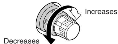
**20 NOISE BLANKER CONTROL [NB LEVEL]** (inner control; p. 5-15)
