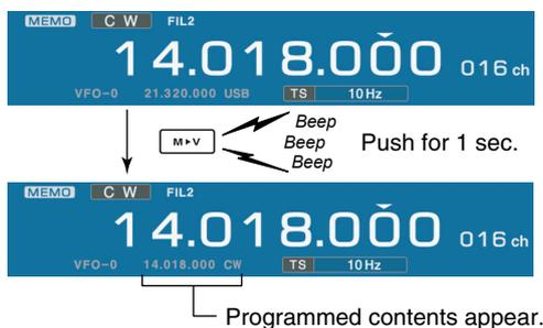
The frequency and operating mode in a memory channel can be transferred to the VFO. Frequency transferring can be performed in either VFO mode or memory mode.
