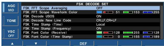
This set mode is used to set the decode USOS function, time stamp setting, etc.
