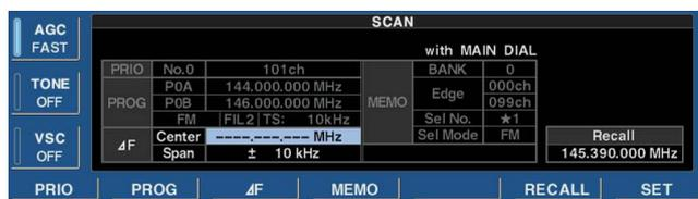
$\Delta F$  scan scans a small range of frequencies around an operating frequency.  $\Delta F$  scan center frequency can be set as specific frequency or as the operating frequency.
