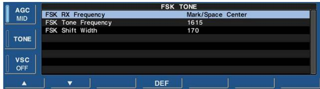
Select the FSK tone frequency and adjust the FSK shift width.
