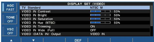
This set mode is used to set the HSB (Hue, Saturation, Brightness) color setting for video input or output, etc.
