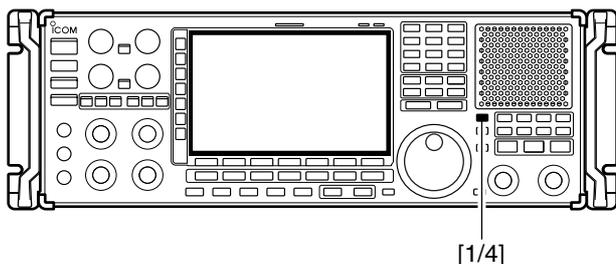
When operating in CW or FSK, the 1/4 tuning function is available. Dial rotation is reduced to 1/4 of normal speed when the 1/4 tuning function is ON for finer tuning control.
