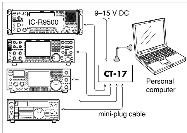
The receiver can be connected through an optional CT-17 CI-V LEVEL CONVERTER to a PC equipped with an RS-232C port. The Icom Communications Interface-V (CI-V) controls the receiver.
