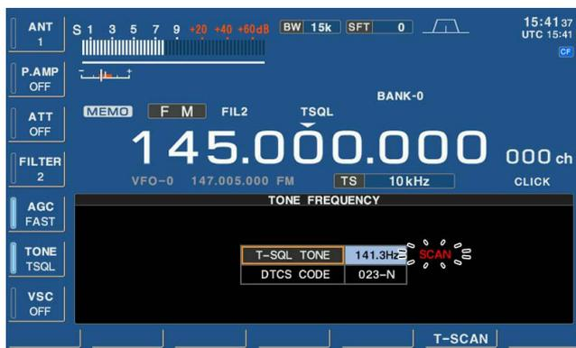
The receiver can detect subaudible tones or the DTCS code in a received signal. By monitoring a signal that is being operated with tone or DTCS squelch function, you can determine the tone frequency or DTCS code necessary to open a squelch.
