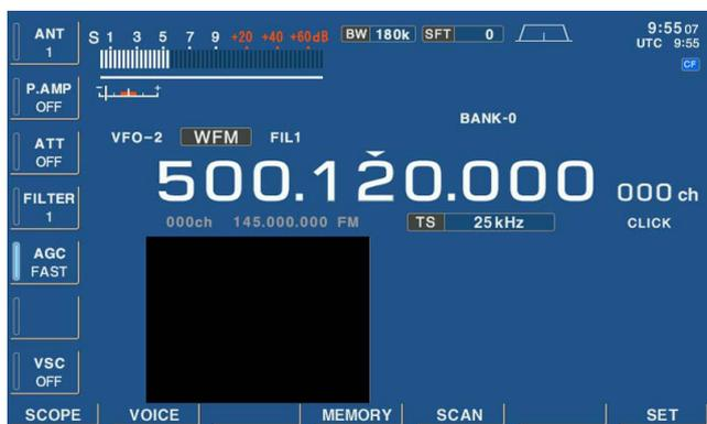
A TV tuner is built-in to the IC-R9500, and connects to the [VIDEO IN] and [VIDEO OUT] on the rear panel using a TV jumper cable to monitor the TV programs (except for USA version).
