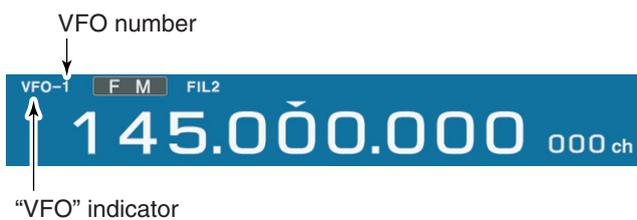
VFO is an abbreviation of Variable Frequency Oscillator, and is commonly referred to as a main tuning function. Frequency, mode and other receiver settings are stored as a set of VFO data.
