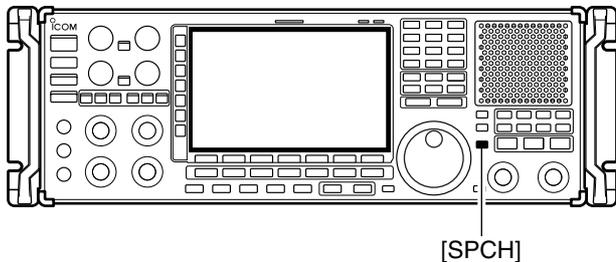
The IC-R9500 has a built-in voice synthesizer to announce the frequency, mode, etc. (S-meter level can also be announced—p. 11-10) in clear, electronically-generated voice, in English (or Japanese).
