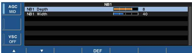
To deal with various type of noises, attenuation level and noise width can be set in NB set mode. Two of noise blanker, NB1 and NB2, can be set independently.
