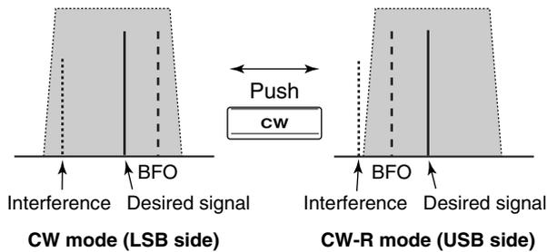
CW-R (CW Reverse) mode uses the opposite side band to receive CW signals.
