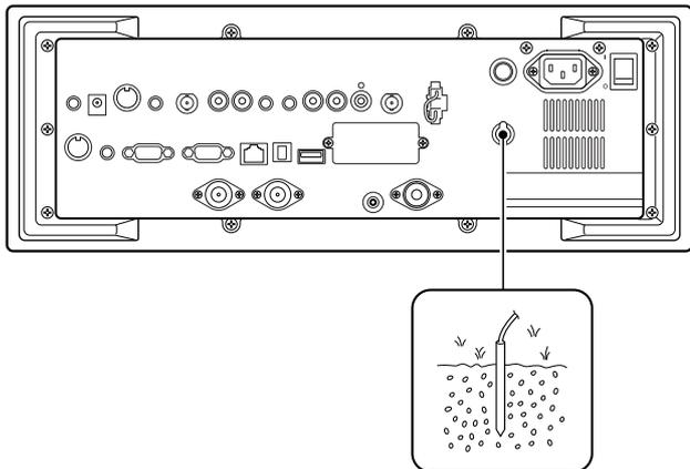
To prevent electrical shock, television interference (TVI), broadcast interference (BCI) and other problems, ground the receiver through the GROUND terminal on the rear panel.
