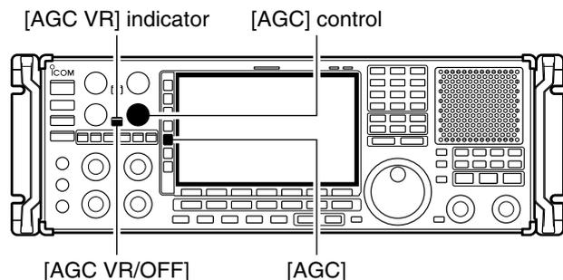
The AGC (auto gain control) controls receiver gain to produce a constant audio output level even when the received signal strength varies greatly.
