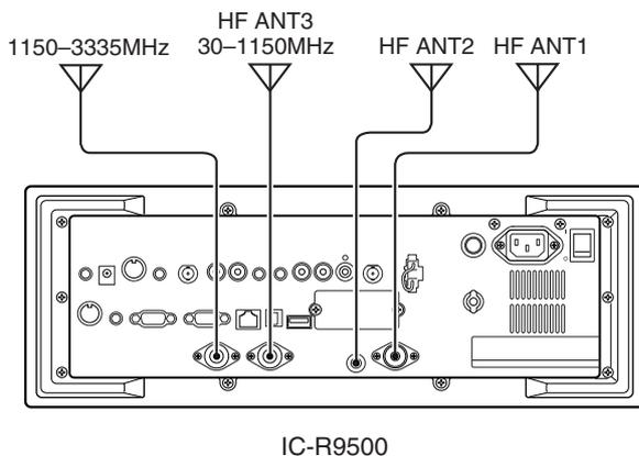
The IC-R9500 has 3 antenna connectors for bands below 30 MHz which are [HF ANT1], [HF ANT2] and [ANT1/HF ANT3]. And antenna control voltage is also output from [ANT SEL] connector for using external preamplifier or antenna selector.
