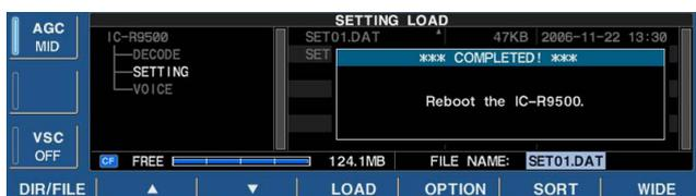
By loading the saved setting file from the CF memory card or USB-Memory, you can easily set up another IC-R9500—several operators settings can easily be applied to one IC-R9500.
