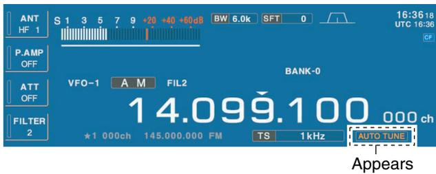
➔ Push [AUTOTUNE] (AFC) to toggle the autotune function ON or OFF.
