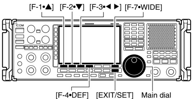
This set mode is used to set the waveform color, center frequency indication for center mode, etc.
