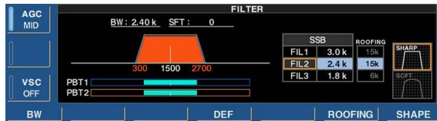
The type of DSP filter shape for each SSB, SSB data and CW can be selected independently from soft and sharp.
