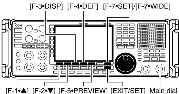
The IC-R9500 has a screen saver function to protect the LCD from the “burn-in” effect.
