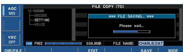
Memory channel contents, set mode settings, etc. in CF card or USB-Memory can be copied between memory devices for backup.
