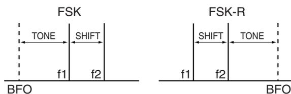
Received characters are occasionally garbled when the received signal has Mark and Space tones reversed. This reversal can be caused by incorrect TNC connections, setting, commands, etc. To receive reversed FSK signals correctly, select FSK-R mode.
