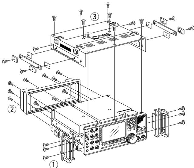
Follow the case opening procedures shown here when you want to install the optional unit UT-122, or replace the clock battery or internal fuse.
