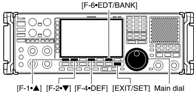
Setting bank limit function for memory channel selection, for memory scan can be set in bank set mode or programming bank name.
