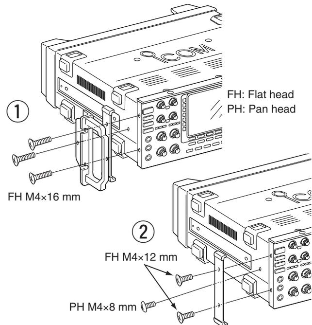
When removing the rack mounting handles, use the supplied screws for attach the side plates.
