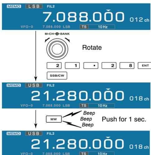
Memory channel programming can be performed either in VFO mode or in memory mode.
