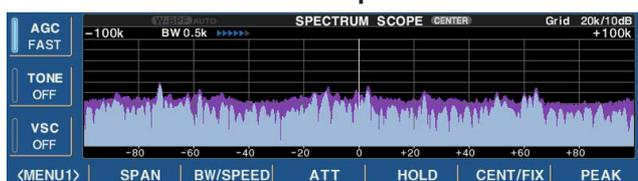
This DSP-based spectrum scope allows you to display the conditions on the selected band, as well as relative strengths of signals. The IC-R9500 has two modes for the spectrum indication— one is center mode, and another one is fixed mode.
