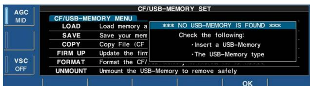
/// **NOTE:** If no USB-Memory is inserted and [F-7•USB] is selected as in step ②, an error message appears.
