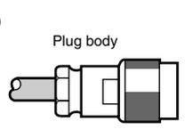
Carefully slide the plug body into place aligning the center conductor pin on the cable. Tighten the nut onto the plug body.
