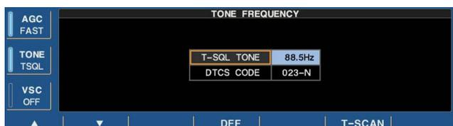
The tone or DTCS squelch opens only when receiving a signal containing a matching subaudible tone or DTCS code. You can silently wait for calls from group members using the same tone.
