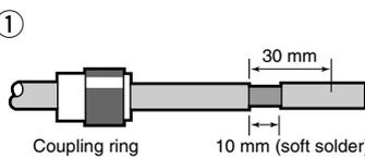
Slide the coupling ring down. Strip the cable jacket and tin the braid.
