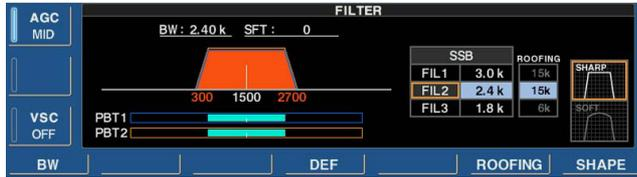
The IC-R9500 has 3, 6 15 and 50 kHz roofing filters at the 1st IF frequency. The roofing filter provides interference reduction from nearby strong signals.
