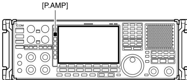
During 1150–3335 MHz (ANT2) operation, either the preamplifier or attenuator is activate exclusively.
