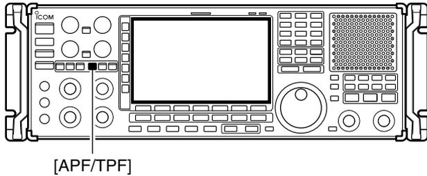
The APF changes the audio frequency response by boosting a particular frequency to enhance a desired CW signal.
