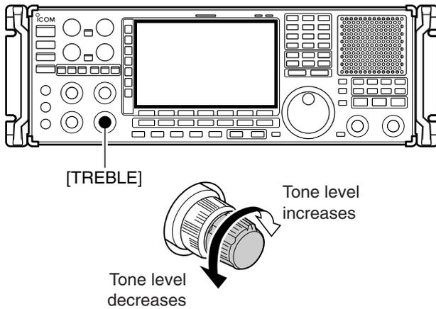
➤ Rotate [TREBLE] control clockwise to increase, counterclockwise to decrease the treble level of the audio tone.
