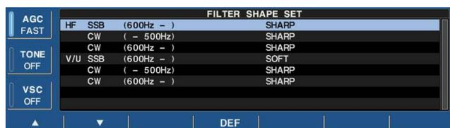
The type of DSP filter shape for each SSB and CW can be selected independently from soft and sharp.
