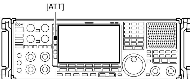
The attenuator prevents a desired signal from being distorted by a very strong signals are near the desired frequency or when very strong electric fields, such as from broadcasting stations, are near your location.
