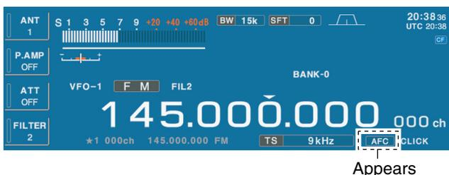
➔ Push [AFC] to toggle the AFC function ON or OFF.
