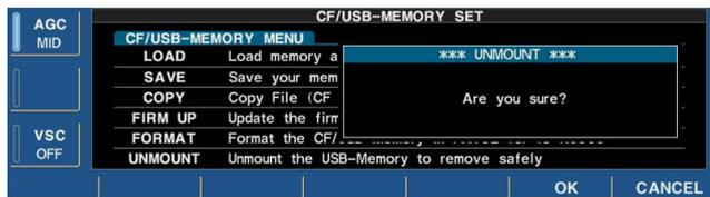
**CAUTION!** When removing the USB-Memory, unmount operation is necessary. Unless otherwise inside data of USB-Memory may be damaged.
