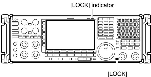
The dial lock function prevents frequency changes by accidental movement of the tuning dial. The lock function electronically locks the dial.
