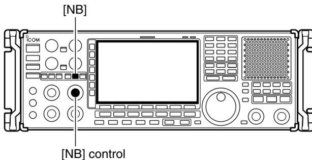
The noise blanker eliminates pulse-type noise such as the noise from car ignitions. The noise blanker is not available for FM, WFM or P25 mode.
