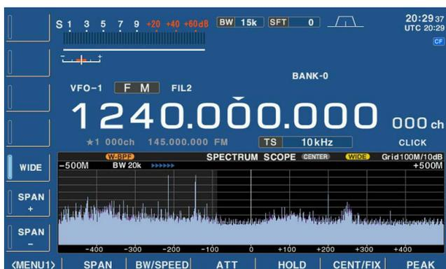
The wide band scope function is available to sweep a wide frequency range (max.  $\pm 500$  MHz). While this function is active, AF monitor is not available.
