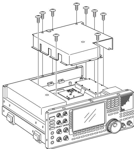
Follow the case opening procedures shown here when you want to replace the internal fuse or optional UT-122 installation.
