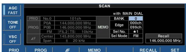
All memory channels (except skip channels) in the selected bank are scanned at up to 40 ch/sec.
