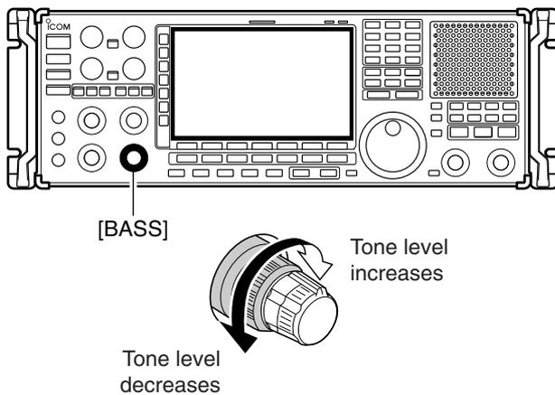
➤ Rotate [BASS] control clockwise to increase, counterclockwise to decrease the bass level of the audio tone.
