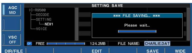
Memory channel contents, set mode settings, etc. can be saved into the CF (Compact Flash) memory card or USB-memory for backup.
