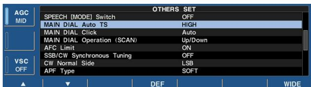
When rotating the main dial rapidly, the tuning speed accelerates automatically.
