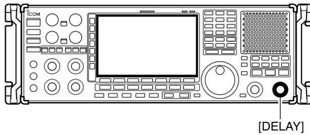
➡ Rotate [DELAY] to adjust the scan pause time when the scan resume setting is set to 'DELAY.'
