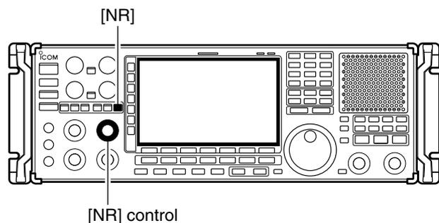
The noise reduction function reduces random noise components and enhances desired signals which are buried in noise. The DSP performs the random noise reduction function.
